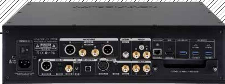
**ABOVE:** Optional Wi-Fi and HDD storage options are hosted alongside digital coax, optical and AES/EBU inputs, USB-B and three USB-A (two for external drives plus one on the fascia) and wired Ethernet. Outputs include balanced XLR and single-ended RCAs alongside digital on coaxial, optical and AES/EBU
