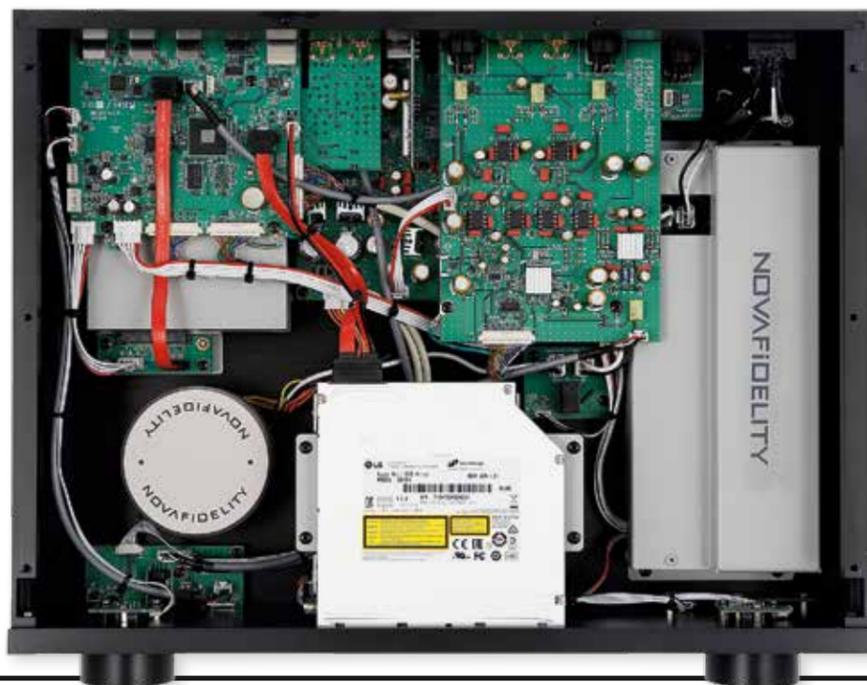
**RIGHT:** The network solution [top left], music library HDD [underneath] and CD ripper [DVD writer, middle] are all powered by a screened switchmode PSU [far right] while the ES9038 DAC/analogue board [top right] has a linear PSU
