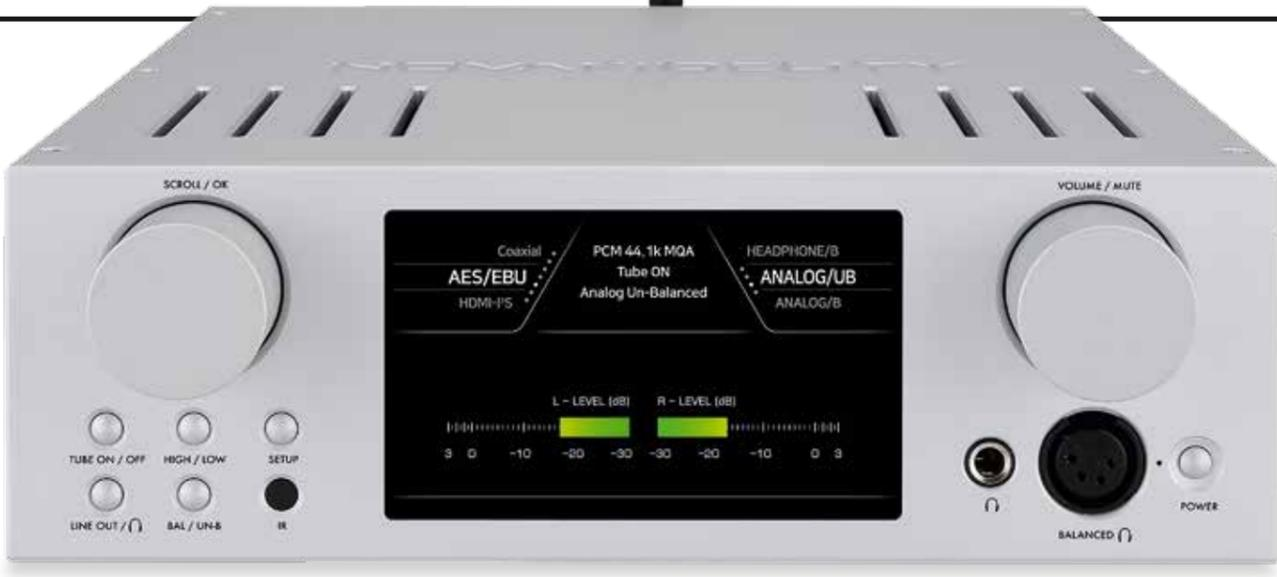
jack socket and an XLR balanced feed, with a choice of ‘High’ or ‘Low’ impedance settings to suit a wide range of headphones [see PM's Lab Report, p67]. In ‘High’ mode the HA500H claims up to 1100mW, and 450mW in ‘Low’, both into 16ohm via the unbalanced headphone output.
