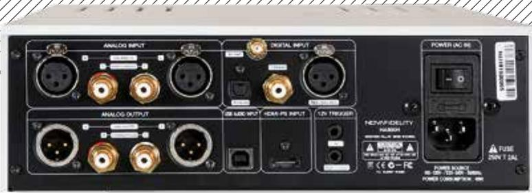
**ABOVE:** Digital inputs span S/PDIF (coaxial, optical), AES/EBU (on XLR), USB-B for computer connection, HDMI for I²S, and wireless Bluetooth. Analogue inputs and fixed/variable analogue outputs are on RCAs and balanced XLRs
