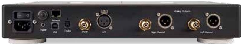
**ABOVE:** All digital inputs are supported here including wired Ethernet (as a DNLA compatible network player the M3 handles up to 384kHz PCM and DSD128 as DoP), USB-B (also 384kHz PCM and DSD128 as DoP), optical/coax S/PDIF and AES/EBU (XLR)
